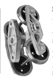
Modern design of bogie used on BR brake fitted wagons 1960 onwards.
