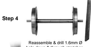
Reassemble & drill 1.6mm Ø hole down & through stretcher, aligning all holes.
